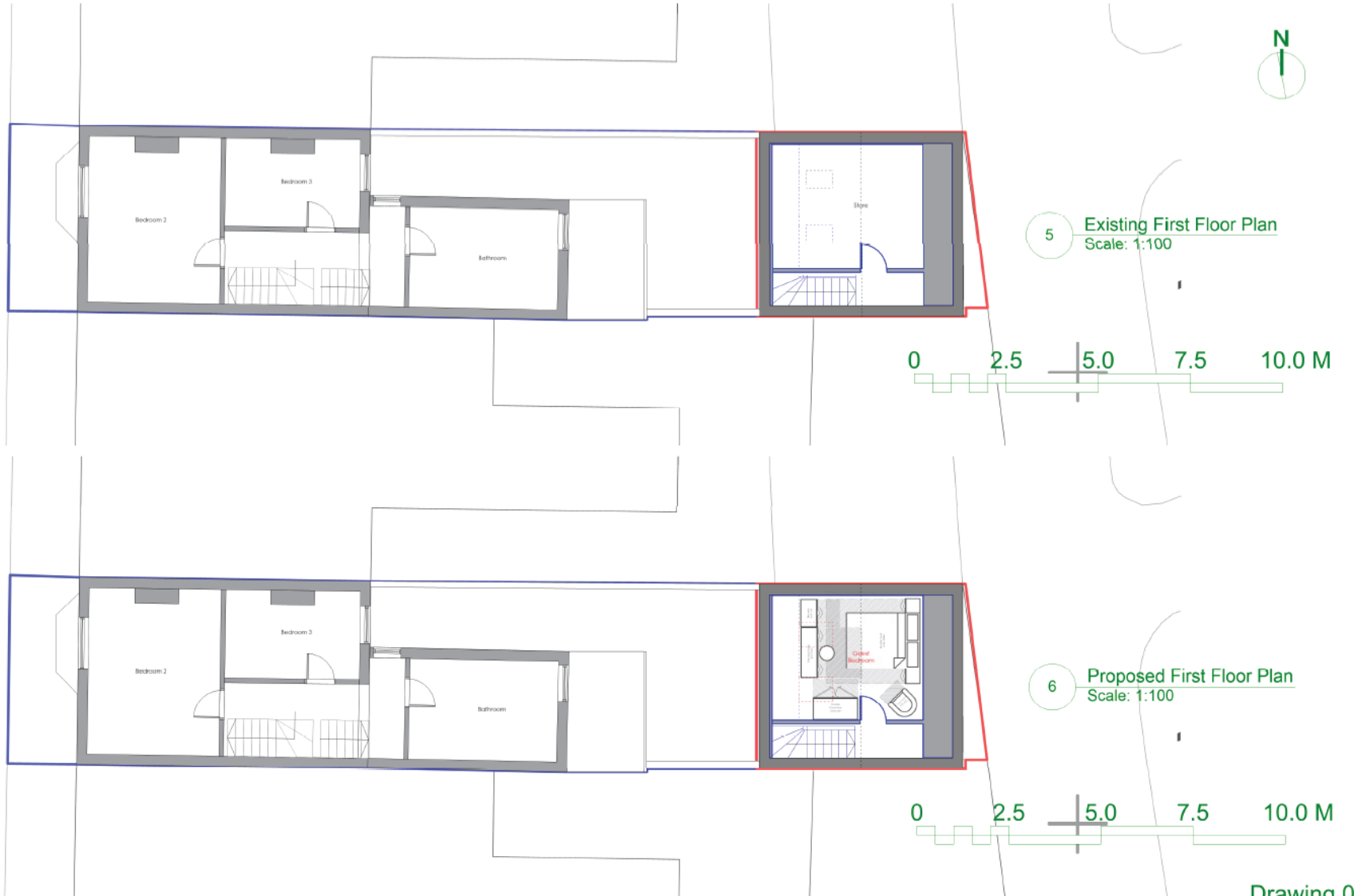
Drawing 003 Existing and Proposed First Floor Plans 1:100 @A3 Alterations to Rear of 41 Milton Street, York, YO10 3EP
